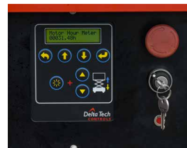
LCD screen, used to display fault code and adjust parameters
