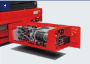
Hydraulic and electric system
